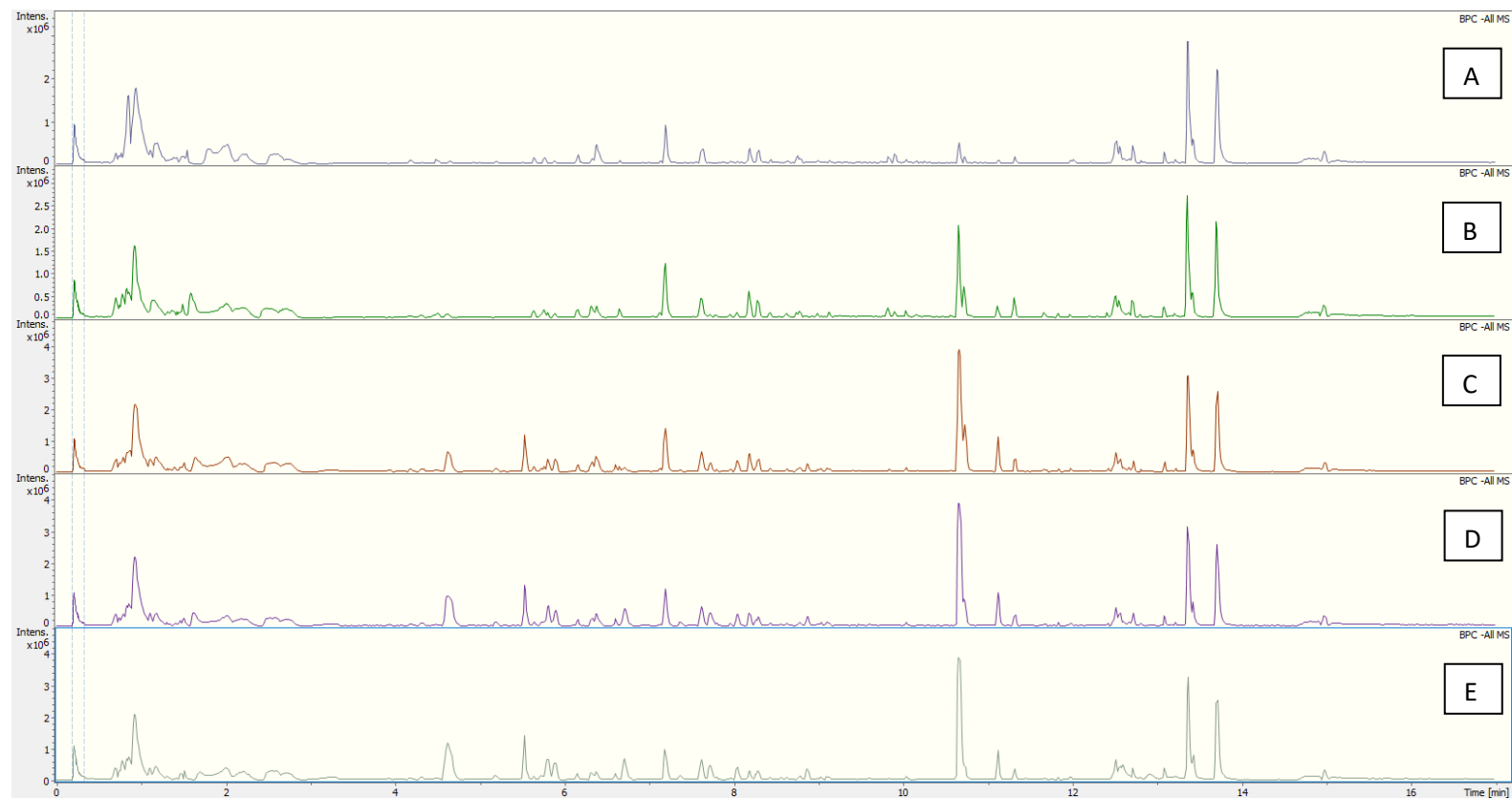
Figure S4. RP-LC-TIMS-TOF MS total ion chromatograms (TICs) in ESI - , of samples from the same vinification protocol, collected at different vinification stages: i) intermediate point of fermentation (A), ii) end of fermentation (B), iii) end of maturation (C), iv) three months of aging (D) and v) six months of aging (E)
